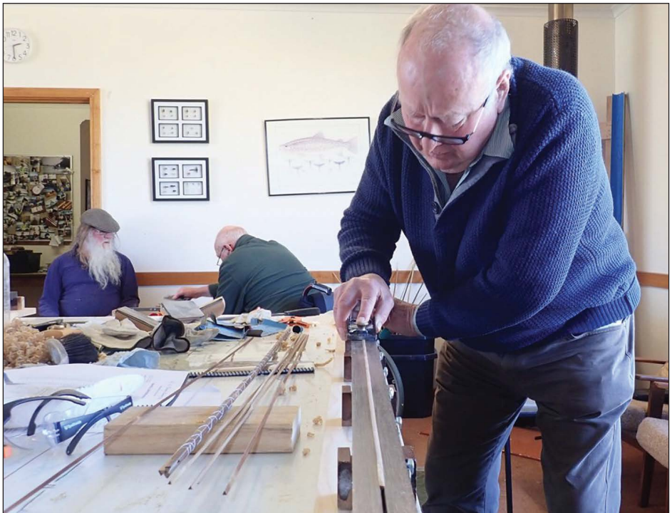
Careful does it – planing the sections for a new rod
